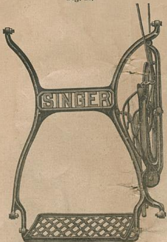
The New Singer Stand Brace (with Belt Thrown Off).—Patented
