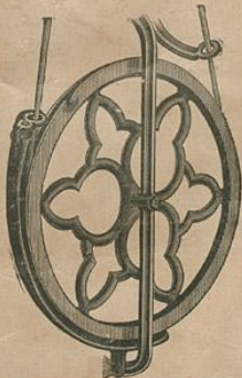
The New Singer Belt Shifter.—Patented
